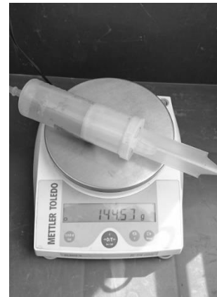
Figure 8. Doser and digital scale with precision 0.01 g.
