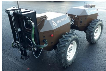
Figure 2. Articulated steering UGV platform prototype with soil sampling mechanism.
