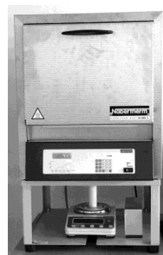
Figure 1. Measurement equipment consisting of furnace Nabertherm L9/11/SW/P330 type and laboratory scales Kern.
