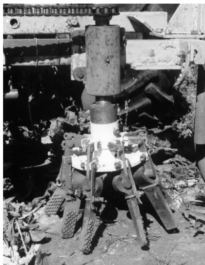
Figure 2. Working head for cleaning root crowns from haulm residues mounted on tractor during experimental investigations.
