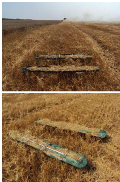
Figure 1. Determination of losses after the passage of a combine on an area of 1 m 2 .
