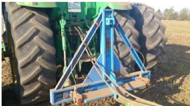
Figure 2. Mechanical part of a measurement apparatus used for measuring of a tension force.
