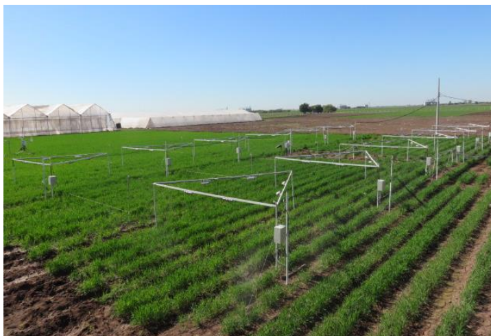
Figure 1. Aerial image of the experimental site where triangular structures were placed containing six thermal radiators each one.
