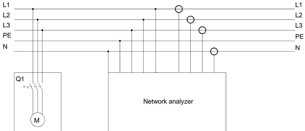
**Figure 1.** Block measurement scheme: L1 to L2 – phases of three-phase TN-S distribution system; PE – Protective Earthing; N – Neutral conductor; Q1 – motor terminal block; M – briquetting press three-phase asynchronous electric motor.
