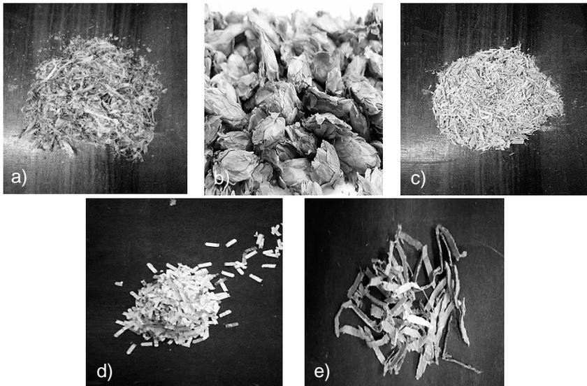
**Figure 2.** Photographs of the used samples. Photographs of the used samples: a) sugar thistle (mouldings); b) hop (natural form – outdoor photography); c) birch (shavings); d) old student book (scrap, fraction 4 x 18 mm); e) carton (scrap, fraction 12 x50 mm).
