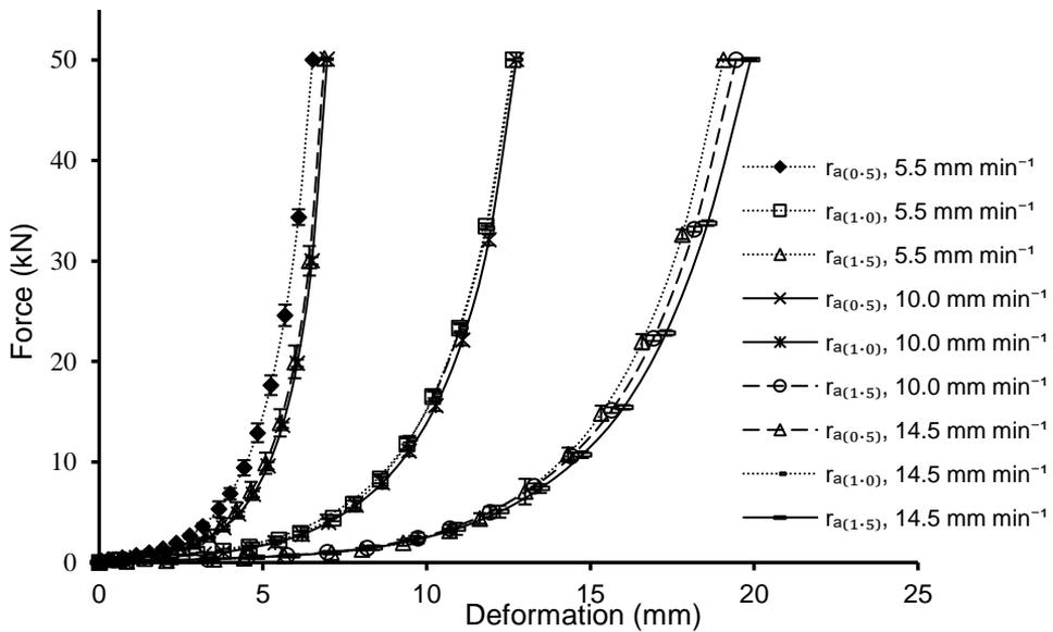
**Figure 2.** Force – deformation profiles of carob powder at applied pressure of 100 MPa, aspect ratios ( $r_a$ ) of 0.5, 1.0 and 1.5 and deformation rates of 5.5, 10 and 14.5 mm min<sup>-1</sup>.
