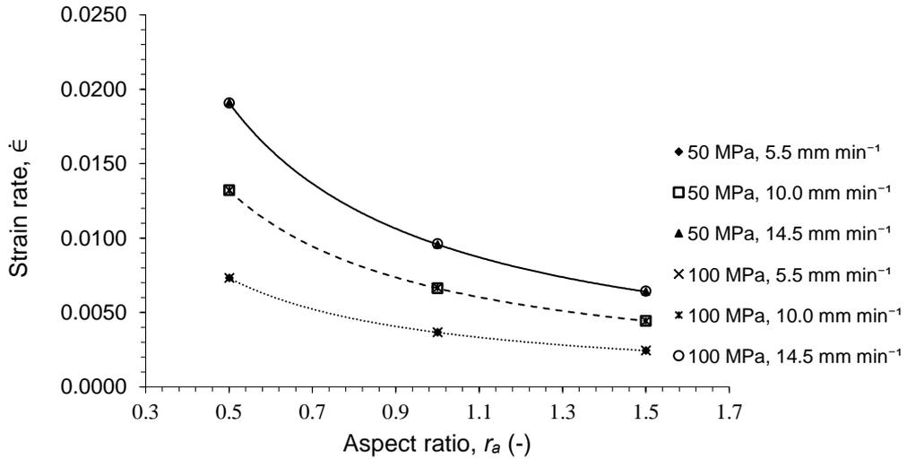
**Figure 3.** Rates of strain in the compressed powder as functions of the aspect ratio at 50 and 100 MPa and deformation rates of 5.5, 10.0 and 14.5 mm min<sup>-1</sup>.
