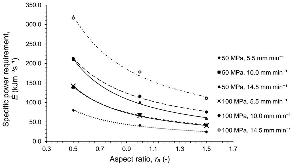
**Figure 4.** Specific power requirement as a function of the aspect ratio, 50 and 100 MPa of applied pressure and deformation rates of 5.5, 10.0 and 14.5 mm min<sup>-1</sup>.
