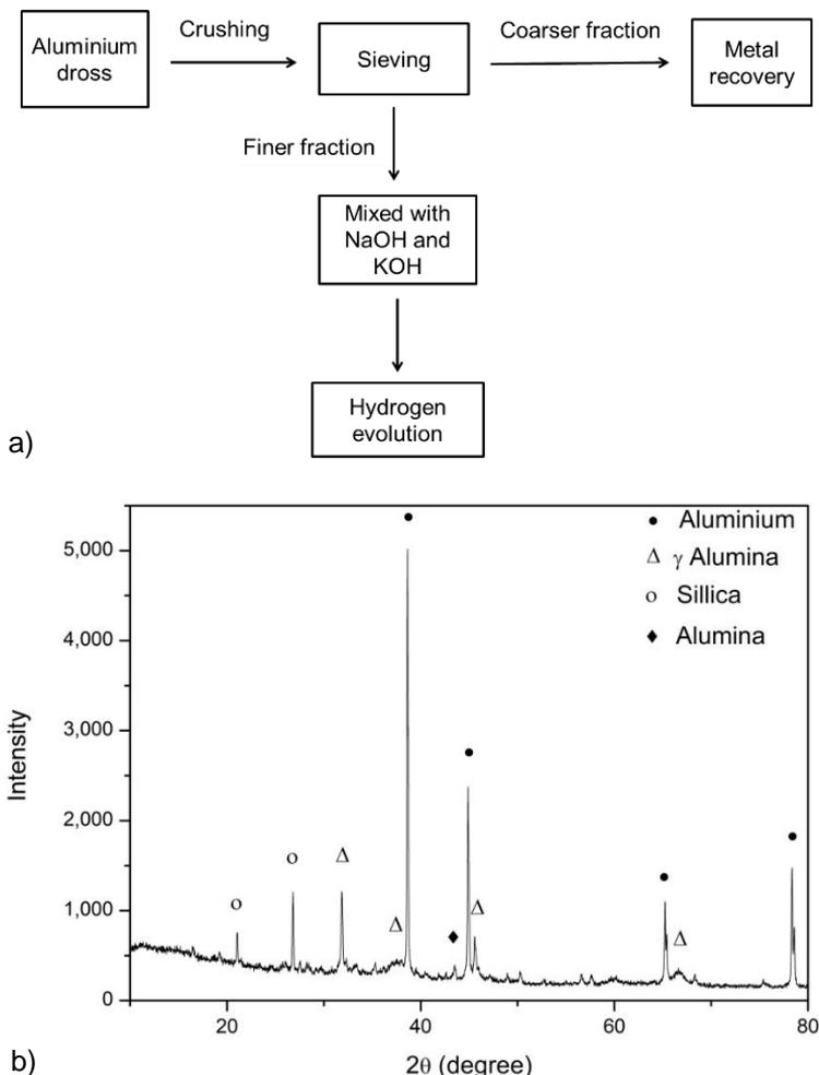
**Figure 1.** a) Schematic diagram illustrating the procedure for hydrogen gas evolution using aluminium dross is shown; b) X-ray diffraction pattern for powdered aluminium dross.
