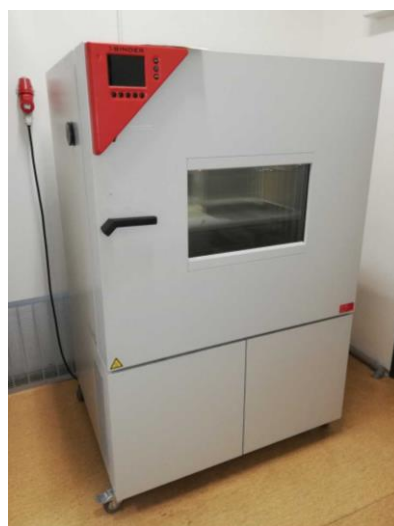
Figure 1. The laboratory programmable chamber MKF240 of the firm Binder.
