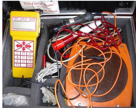
Figure 5. The Great Dane corrosion mapping system.
