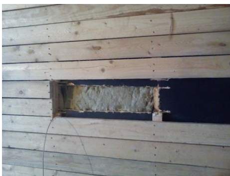
Figure 3. Applying sensors between layers.
