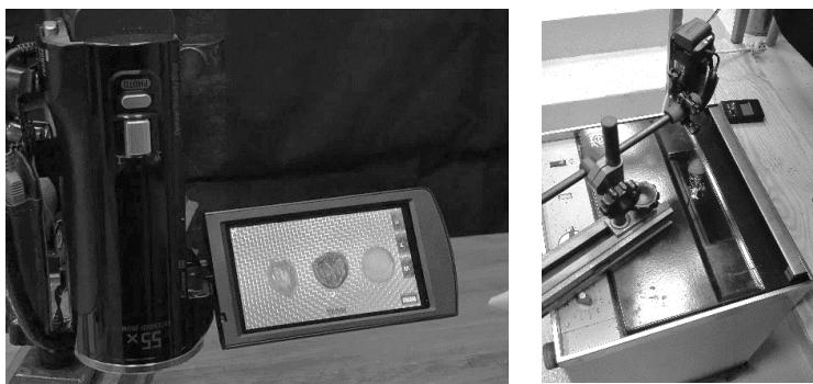
Figure 1. Experimental drying oven equipped with HD camera.
