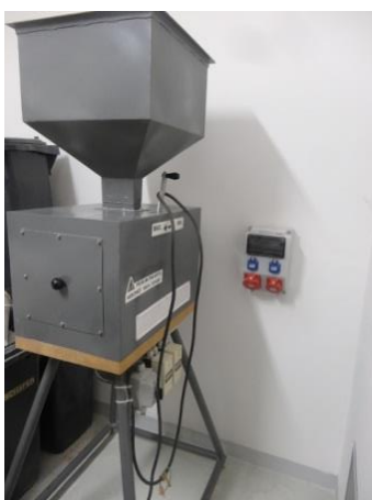
Figure 1. Two roller mill VKM 130/150.
