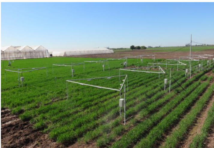
Figure 1. Aerial image of the experimental site where triangular structures were placed containing six thermal radiators each one.
