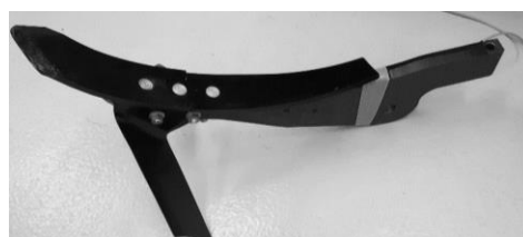
Figure 2. The tool module is ready for installation on the test machine.
