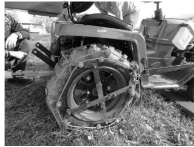
Figure 5. The test tractor Mini 070 type equipped with the special driving wheels.
