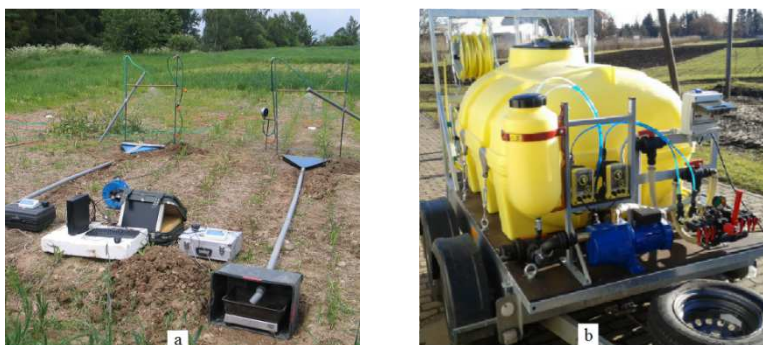
Figure 1. Field experiment (a), rainfall simulator developed on CULS in Prague (b).
