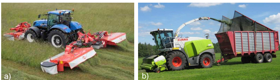
Figure 6. n (a) Triple gang mower of the type envisaged for 9- and 12-m systems. In (b) Example of a self-propelled harvester loading into a towed trailer.
