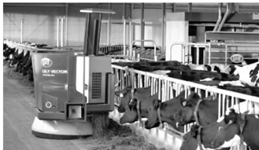
Figure 2. Automatic feeding system Lely Vector (Source: https://www.agropartner.cz/automatizky-system-krmeni-lely-vector-p255.html ).
