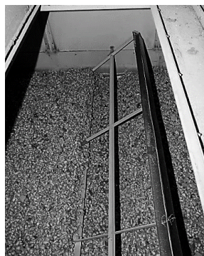
Figure 2. Rotor installed above the first belt of belt dryer.
