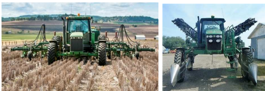
Figure 3. A 8400-series John Deere CTF-compatible tractor (left) with front and rear axles extended to 3-m. Note the tractor positioned on the permanent traffic lanes of a 9-m module CTF system in no-tillage. The machinery width ratio is 3:1, that is, 9-m front combine harvester and planter bar, and 27-m boom width sprayer (right), also with both axles extended to 3-m.
