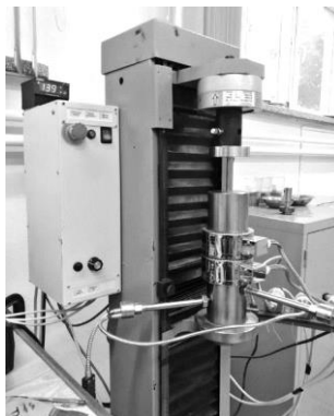
Figure 2. Testing stand for agglomeration process.
