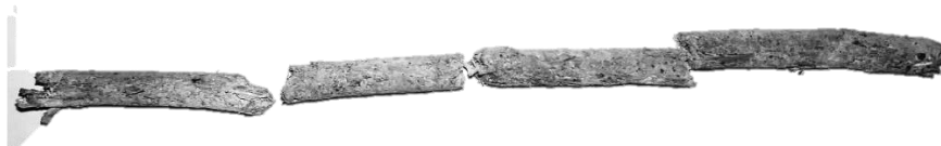
Figure 7. Pellets made of digestate with 20% of calcium carbonate.
