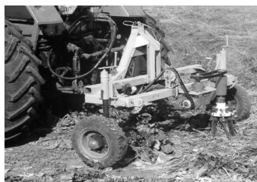
Figure 2. An experimental installation – a cleaner of the root crop heads from the haulm residues.
