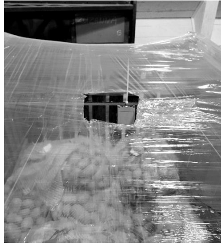
Figure 4. Datalogger placement in a storage box.
