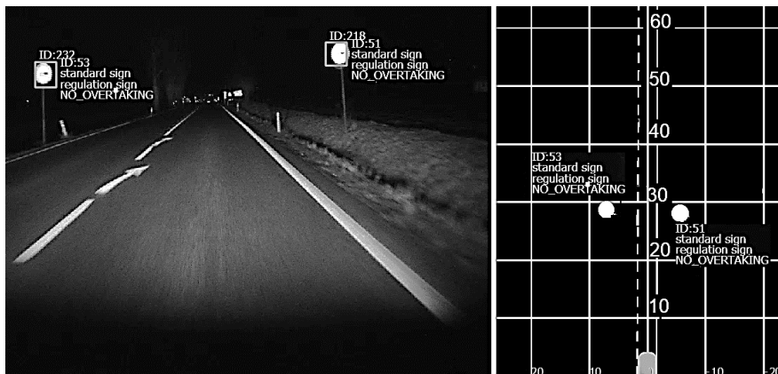
Figure 4. The screen view of two visualization filters of ADTF. (Left) Video widget with the filter of recognition all traffic signs. (Right) Coordinate graph for determining RD of the signs. Source: ADTF development environment.
