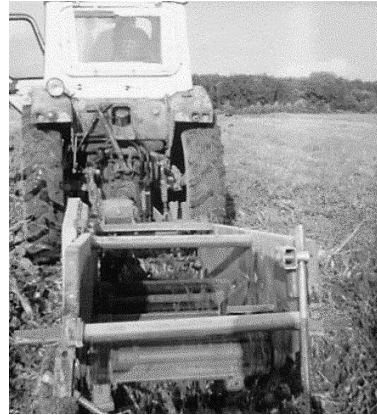
Figure 6. General view of experimental unit with mounted spiral-type potato cleaning unit.
