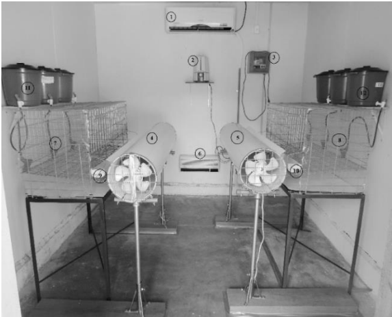
Figure 1. Inside view of the climatic chambers, where 1 – air conditioning; 2 – air humidifier; 3 – electronic temperature and relative humidity controller (MT-531R plus); 4 and 5 – ventilation tubes; 6 – air heater; 7 and 8 – cages; 9 and 10 – feeders; 11 and 12 – water tanks.
