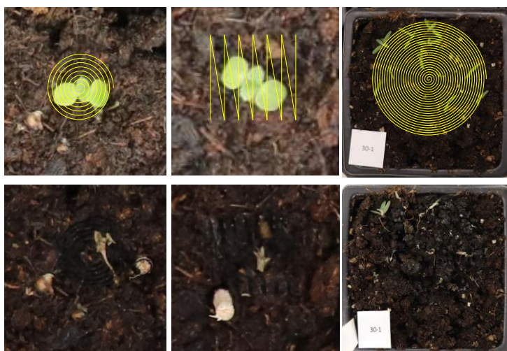
Figure 2. Laser movement patterns used during plant treatment: upper row – individual plant spiral, individual plant ‘zig-zag’, whole pot spiral; lower row – respective treatment results.
