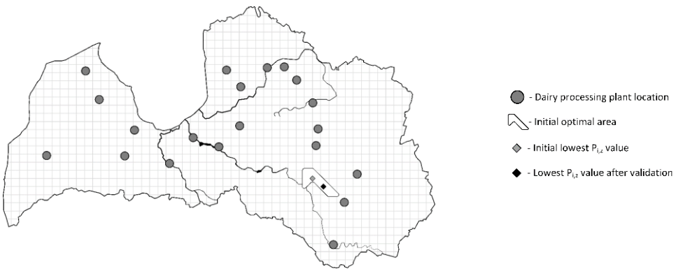
Figure 4. Optimization model repeated with halved XY axis resolution: i = \{0...53\} ; z = \{0...32\} . Initial optimal area (white area) was located by marking 10 coordinates with the lowest P_{i,z} values. Grey square – lowest initial P_{i,z} value.
