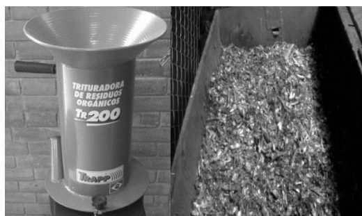
Figure 5. Organic material crusher (left) and plant material disposed in the reactor (right).
