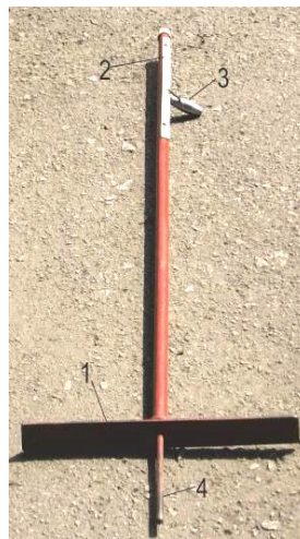
Figure 5. Instrument for measuring tillage depth: 1 – cross bar; 2 – measuring scale; 3 – lever; 4 – rod.
