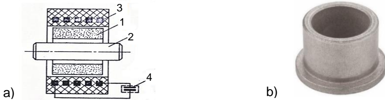
Figure 3. The scheme of magnetic pulse pressing of the bushings (a) and the sample sleeve with a shoulder: 1 – powder; 2 rod; 3 – inductor; 4 – pulse current generator.
