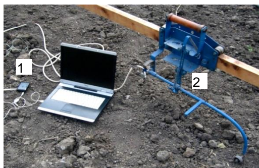
Figure 4. Device for measuring field profile oscillations: 1 – Arduino Uno; 2 – profilometer.
