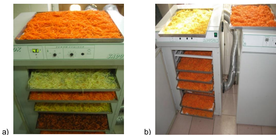
Figure 2. A general view of the convective dryer: a) carrot quantities prepared and loaded into the dryer's chamber; b) dried carrot quantities.
