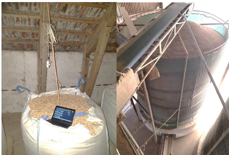
Figure 1. The storage of spelt grain in a FIBC bag (on the left) and in a tower silo with steel wire construction and textile liner (on the right).
