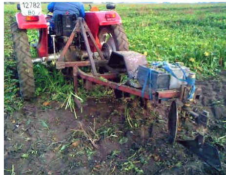
Figure 6. Experimental unit during field study of root crown protrusion above soil surface level.
