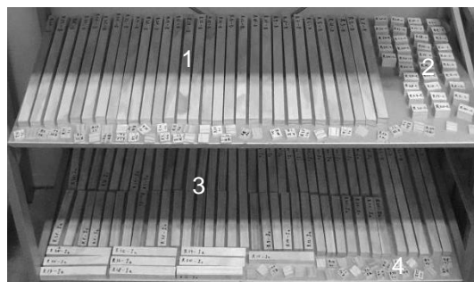
Figure 1. Example of radiata pine specimens: 1 – bending strength and modulus of elasticity specimens 2 – moisture content, density and compression strength specimens; 3 – resistance to impact specimens and 4 – swelling specimens.
