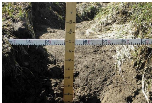
Figure 2. A full-scale study of soil washout products during a period of heavy rainfall.
