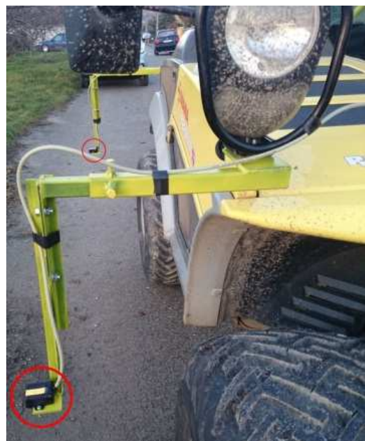
Figure 3. Dislocations of sensors of acceleration on machine (is the same on the hidden part of machine).
