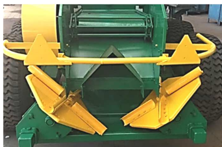
Figure 2. General appearance of prototype fertiliser spreading tools with tilted axes installed in improved-design machine for top dressing with mineral fertilisers.
