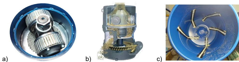
Figure 2. Two machines were used for pelletising: extrusion pelletising: a – working wheel with matrix, b – overall operating diagram of the granulating system. Drum granulation: c – Working rotating cylinder with adjustable angle.
