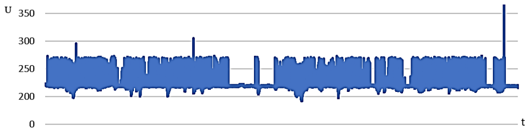
Figure 10. Shock vibration load graph for one working day.
