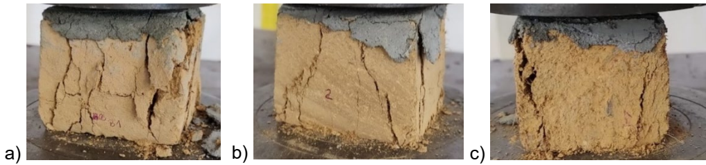
Figure 7. Samples broken after uniaxial compression test: a) reference (0% fiber); b) 1% fiber; and c) 2% fiber.
