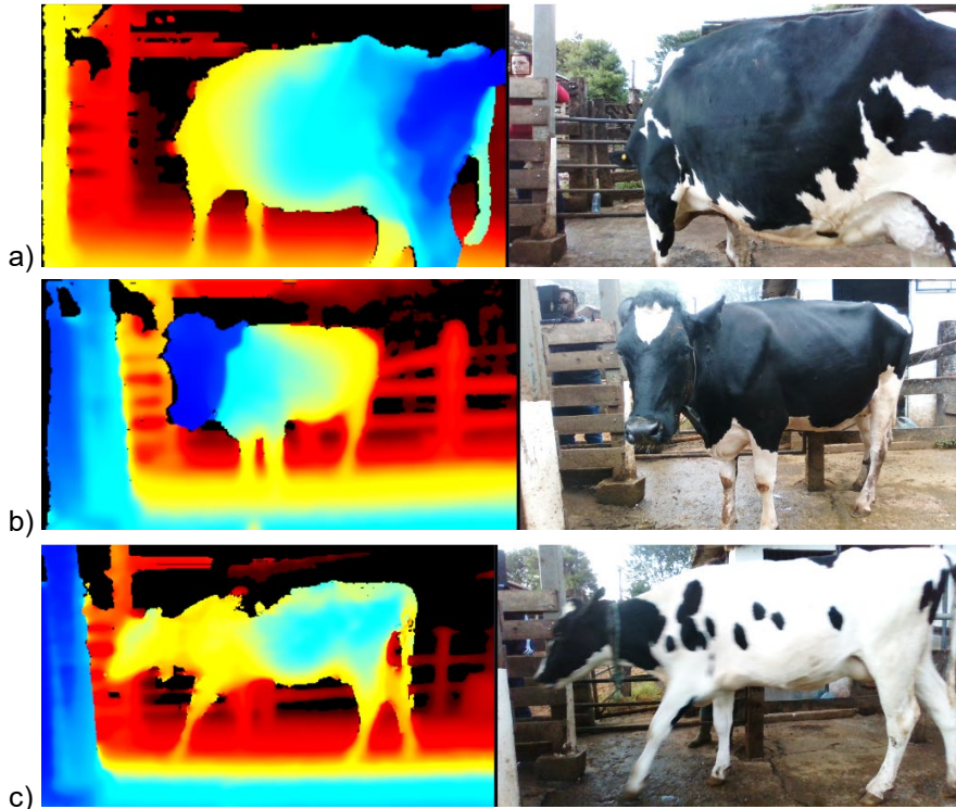
Figure 7. Examples of images rejected for CC measurement, organized in pairs with RGB view (right) and Depth view (left): a) misalignment of the body axis; b) head turned laterally; c) visual distortion caused by light reflection.
