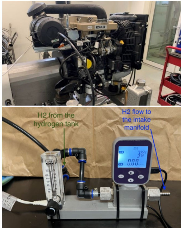
Figure 1. Engine with a test bench and hydrogen flow meter.
