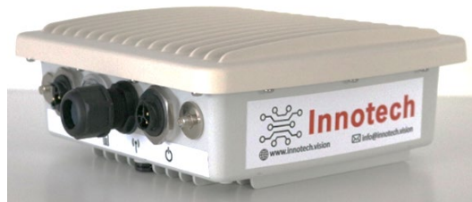
Figure 2. The data processing and communication unit of the WD system before deployment.
