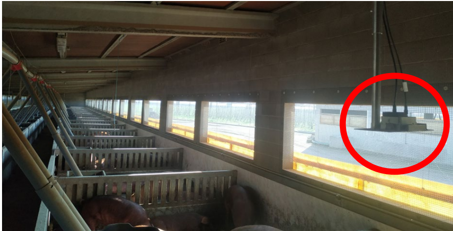
Figure 1. The WD camera installed above the resting area in the pen on a commercial farm in Spain.
