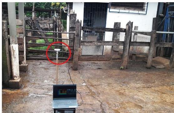
Figure 2. Camera installed to capture side images.
