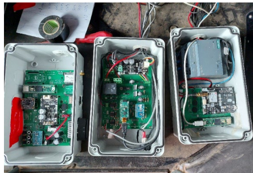
Figure 5. On the left is the 2 nd version with All-in-One board including also GNSS. In the middle is the 1 st version of board. On the right is the 1 st GNSS board and hydraulic electronic control which is linked with Fig. 3 hydraulic control unit.
