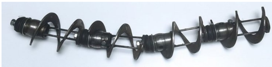
Figure 2. General view of the fabricated flexible sectional screw working body.
