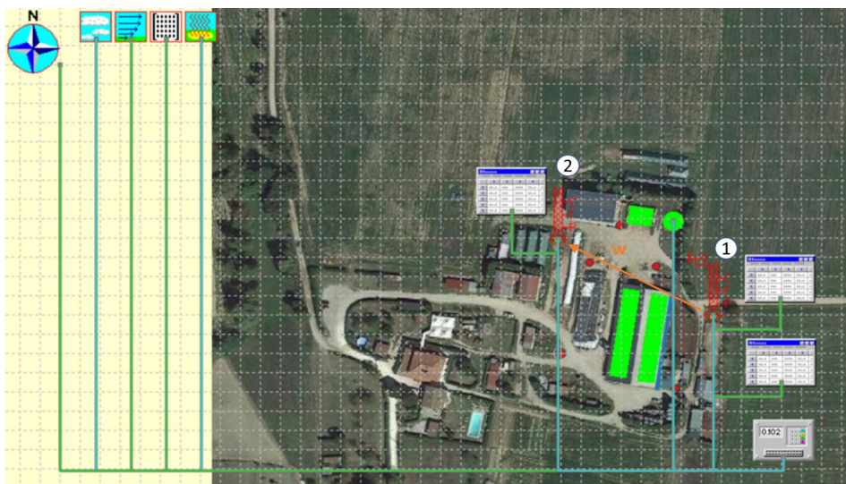
Figure 1. View of the commercial dairy farm (latitude 43.963270°, longitude 11.418885°) and inside the project of the WindTrax software environment. Point 1: upwind G-eko 2.0 multi-sensor unit. Point 2: downwind G-eko 2.0 multi-sensor unit.
