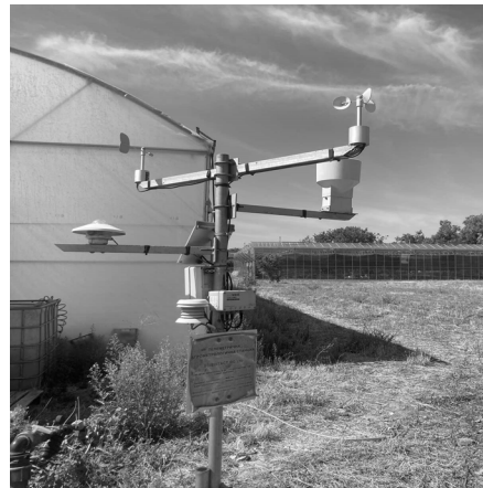
Figure 2. Experimental microclimate monitoring setup consisting of a portable ESP32-based IoT system and a reference Meteobot® weather station used under open-field conditions.
