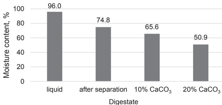
**Figure 3.** Moisture content for different types of digestate.
