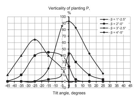
Figure 9. The dependence of planting verticality on the tilt angle of the planting cone  $\beta$ .
