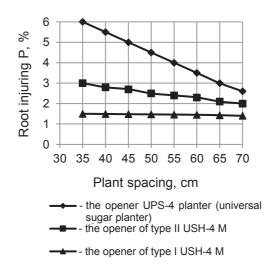
**Figure 2.** The dependence of root injure on the type of the opener.
