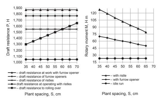
The dependence of the rotary moment on the machine driving shaft upon plant spacing and operating mode is presented in Fig. 13.
