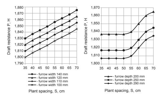
**Figure 10.** The dependence of draft resistance of furrow openers on plant spacing.
