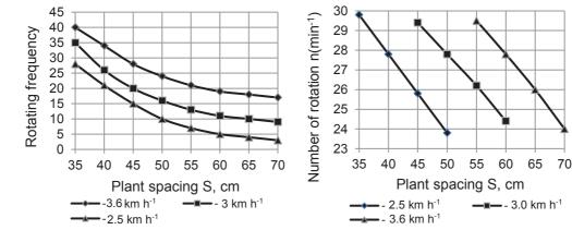
**Figure 4.** The dependence of the planting unit rotating frequency on plant spacing at different tractor gears.
