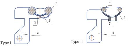
**Figure 1.** The designed openers of planting unit: 1 – metal ring; 2 – porous fixing; 3 – semi-sphere; 4 – hanger.
