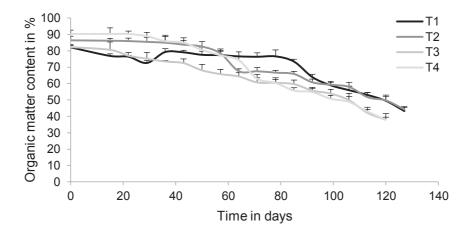
Figure 5. Organic matter evolution during the composting process.
