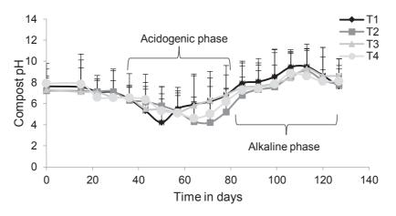
Figure 1. Temporal evolution of pH during composting.
