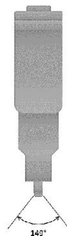
**Figure 1.** Spray angle schematics of the injector nozzles.
