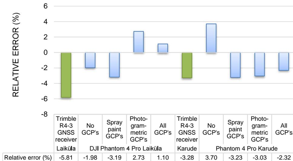
**Figure 6.** Relative errors in the volumes of the models created from the GNSS and DJI Phantom 4 Pro data of Laiküla and Karude objects compared to the results obtained from the laser scanning data (Kokamägi, 2018a).
