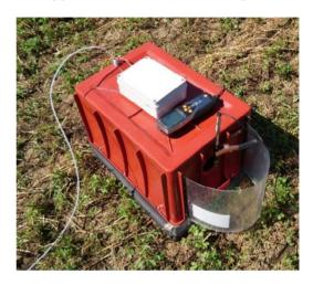
Figure 1. Emissions measuring wind tunnel.
