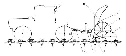
**Figure 1.** Design and process scheme of asymmetric top harvesting unit in longitudinal-vertical plane: I – wheeled tractor; II – trailed asymmetric harvesting machine; 1 – frame; 2 – universal-joint drive; 3 – pneumatic support-and-finder wheel; 4 – rotary haulm cutting device; 5 – conveying device; 6 – loading device.
