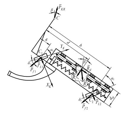
Figure 3. Equivalent diagram of an aggregated harvester.
