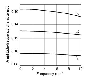
**Figure 4.** Amplitude-frequency characteristic of the course angle  $\varphi$  of the tractor of the integral configuration when it works out disturbances in the form of oscillations of the turn angle  $\beta$  of the mower harvester at different speeds of the machine: 1)  $V_o = 1.5 \text{ m s}^{-1}$ ; 2)  $V_o = 2.0 \text{ m s}^{-1}$ ; 3)  $V_o = 2.5 \text{ m s}^{-1}$ .
