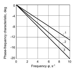
**Figure 5.** Phase-frequency characteristic of the course angle  $\varphi$  of the tractor of the integral configuration when it works out disturbances in the form of oscillations of the tiller turning angle  $\beta$  at different speeds of the machine: 1)  $V_o = 1.5 \text{ m s}^{-1}$ ; 2)  $V_o = 2.0 \text{ m s}^{-1}$ ; 3)  $V_o = 2.5 \text{ m s}^{-1}$ .
