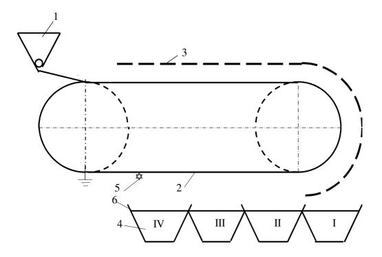
**Fig. 1.** Scheme of the conveyer type electric separator: 1–batcher; 2–conveyer belt (grounded electrode); 3–corona discharge field electrode; 4–reception sizer; 5–brush; 6– partitions between fractions
