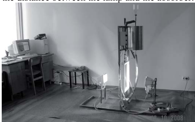
Fig. 3. A stand for investigating the absorber of the solar collector with reflectors.
