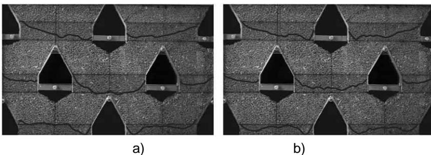
**Figure 3.** Qualitative particle velocity distribution over the vertical cross-section in the bottom part of the dryer: a) at 300ms opening time; b) at 1,000ms opening time.
