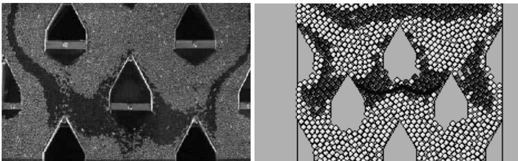
**Figure 1.** Coloured grain layer in the test dryer during discharge and 2D simulation.
