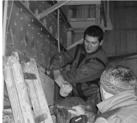
**Figure 6.** Sampling from industrial dryer.
