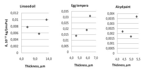
Figure 3. Water vapour permeation coefficient depending on the thickness of layers.
