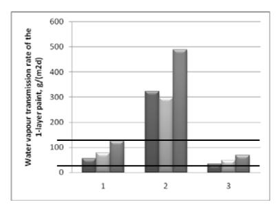
**Figure 2.** Water vapour transmission rate of paints *V*: 1 – linseed oil paint, 2 – egg tempera, 3 – alcyd paint.
