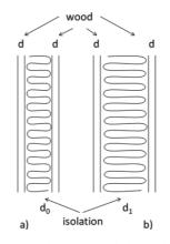
**Figure 1.** Model wall construction: a) original isolation, b) improved isolation.  $d_0 =$ original thickness,  $d_1 =$  thickness of wider insulation, d = thickness of the inner and outer wood wall.
