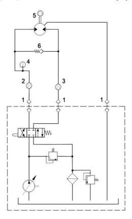
**Figure 6.** Designed hydraulic circuit: 1 -quick couplers, 2 -flowmeter on pressure branch, 3 -flowmeter on waste branch, 4 -thermometer, 5 -optical revolution counter of cutting disc, 6 -one-way valve with spring.
