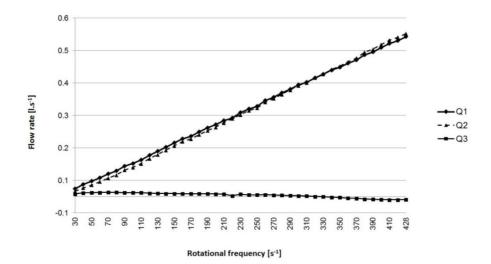
**Figure 7.** Graph of dependancy of hydraulic oil flow on cutting disc rotational frequency: Q1 - hydraulic oil flow in pressure branch, Q2 - hydraulic oil flow in waste branch, Q3 - calculated flow of leakage fluid.
