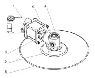
**Figure 2.** Rear transmission with hydromotor: 1 - axial piston hydromotor, <math>2 - coupler, 3 - extension, 4 - angular gear, 5 - carrier, 6 - cutting disc.
