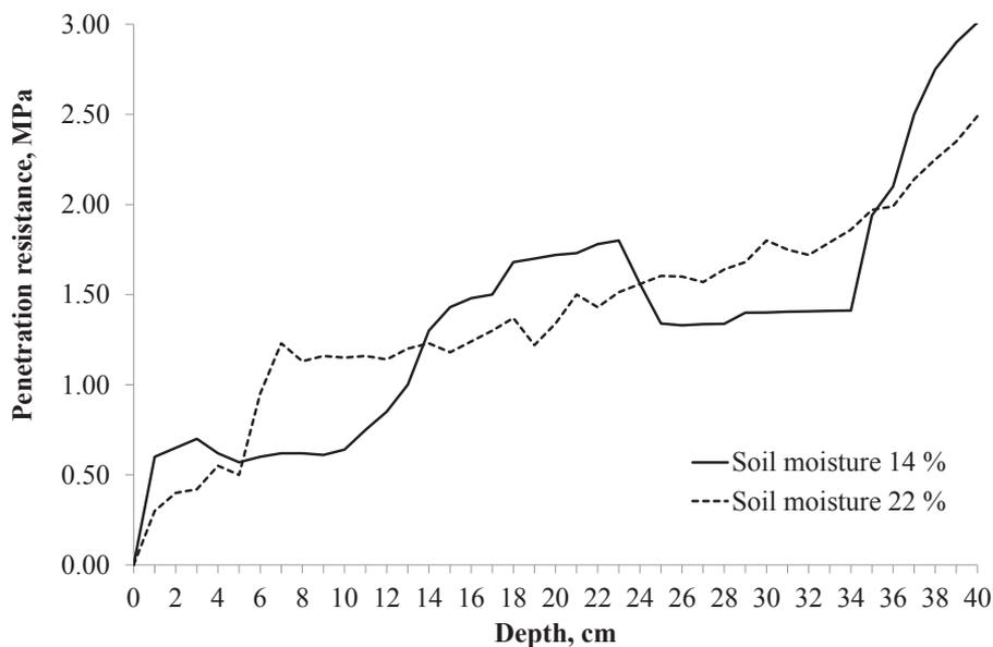
**Figure 4.** Penetrometrical resistance in the same field at diferent soil moisture.
