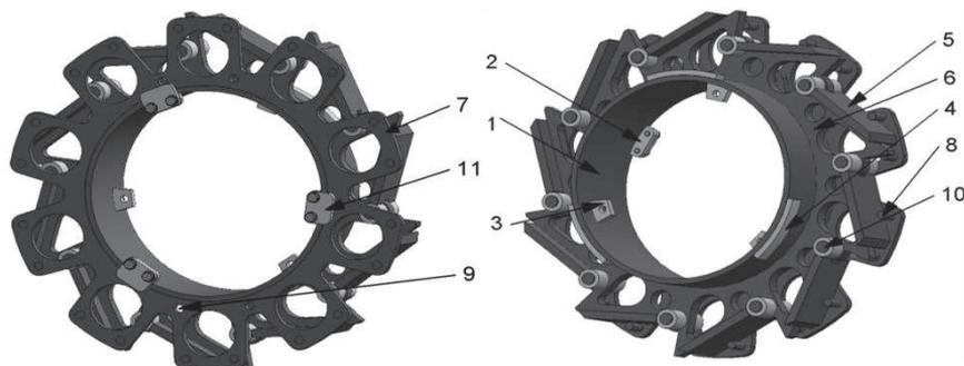
**Figure 1.** Wheels equipped with auto-extensible blades: 1 – support tube, 2 – locking tab, 3 – bracket fastening the mechanism to the wheel disc, 4 – spacer plates, 5 – blade, 6 – driving disc, 7 – blade control disc, 8 – guide pin, 9 – locking hole, 10 – blade pin, 11 – buffer plate.
