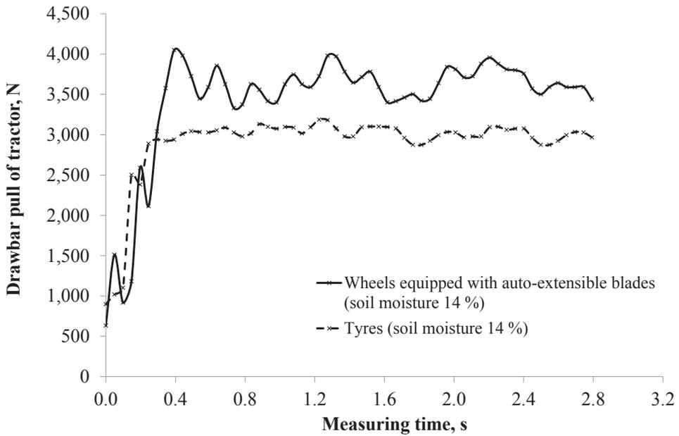
**Figure 5.** The comparison of special wheels and standard tyres on the basis of drawbar pull measured at soil moisture  $w = 14\%$ .
