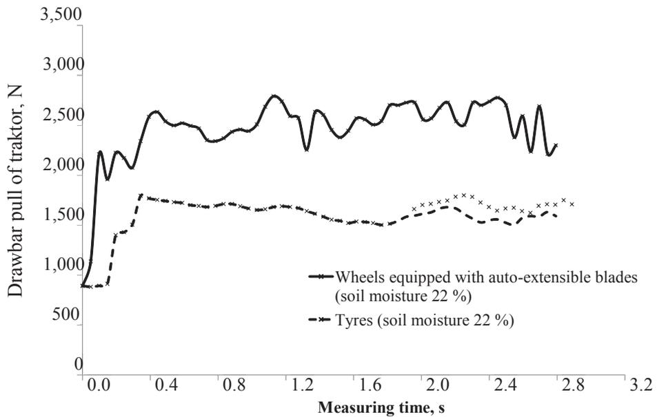
**Figure 6.** The comparison of special wheels and standard tyres on the basis of drawbar pull measured at soil moisture  $w = 22\%$ .
