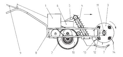
**Figure 1.** Main assemblies and parts of a motoblock-type harvester (Patent EE05488 B1): 1 – engine, 2 – power transmission elements, 3 – picking reel, 4 – conveyor, 5 – chute, 6 – berry box, 7 – copying unit, 8 – frame, 9 – steering levers, 10 – wheels, 11 – reel shaft, 12 – picking rake, 13 – rake tooth, 14 – hook spring-tine.
