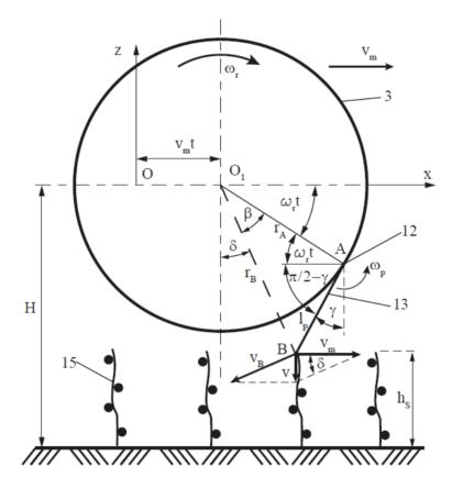
**Figure 2.** Calculation scheme for compiling equations of the trajectory of picking reel's rakes and for determining the height of the picking reel shaft from the ground: 3 - picking reel, 12 - picking rake, 13 - rake teeth, 15 - blueberry plant.
