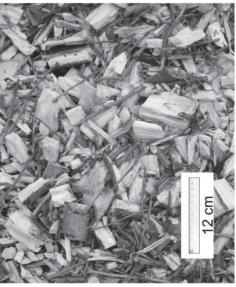
**Figure 5.** Example of wood chips from poplar harvested with the prototype.
