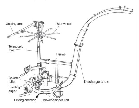
Figure 3. Principle of the ATB mower-chipper unit.
