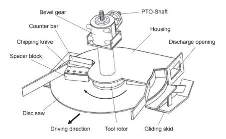
Figure 2. Principle of the ATB mower-chipper unit.
