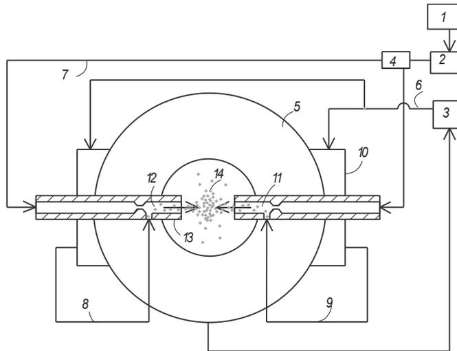
**Figure. 2.** Schematic of the formation of the air-fuel mixture in a pulveriser fuel supply system (Olt et al., 2013). 1 – compressor; 2 – pressure vessel; 3 – fuel tank; 4 – air-pressure regulator; 5 – system corps; 6 – fuel line to fuel-flow regulator; 7 – air line; 8 and 9 – fuel line to pulveriser; 10 – fuel-flow regulator; 11 and 12 – first-step carburation; 13 – pulveriser; 14 – second-step carburation.
