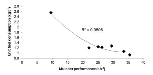
Figure 3. Unit fuel consumption.
