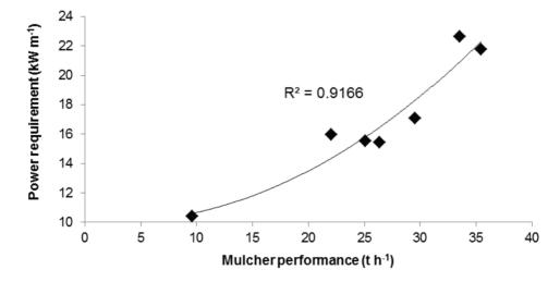
Figure 1. Mulcher power requirement.
