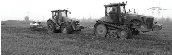
**Figure 1.** The measuring set during the measurement of tensile force using the tensile dynamometer LUKAS type S-38.
