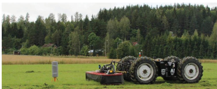
Figure 4. Test setup, an artificial obstacle representing an electricity pole.
