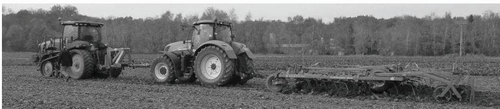
Figure 1. Measuring set. From left: pulling tractor John Deere 8320RT, measuring frame, measuring stick, pulled tractor New Holland T7050 for lifting and lowering of the cultivator, cultivator Köckerling Gruber Vario with 5 m working width.
