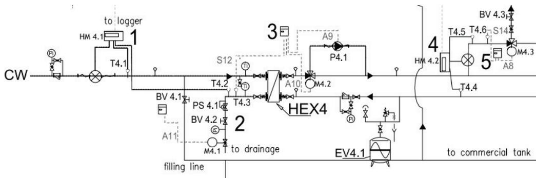
**Figure 3.** Domestic hot water load imitation diagram (1 – flow rate and power meter for cold side; 2 – pressure valve; 3 – controller for imitating DHW load; 4 – flow and power meter for test tank; 5 – controller for test tank return option).
