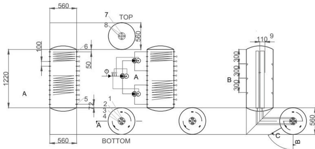
**Figure 4.** Experimental tank's inlet/outlet elements (1 – hot water from solar collector; 2 – supply to DHW; 3 – return to solar collector loop; 4 – return from heating load; 5 – cold water supply; 6 – supply to heating load and DHW; 7 – bleeding valve; 8 – spare fittings; 9 – stratification pipe).
