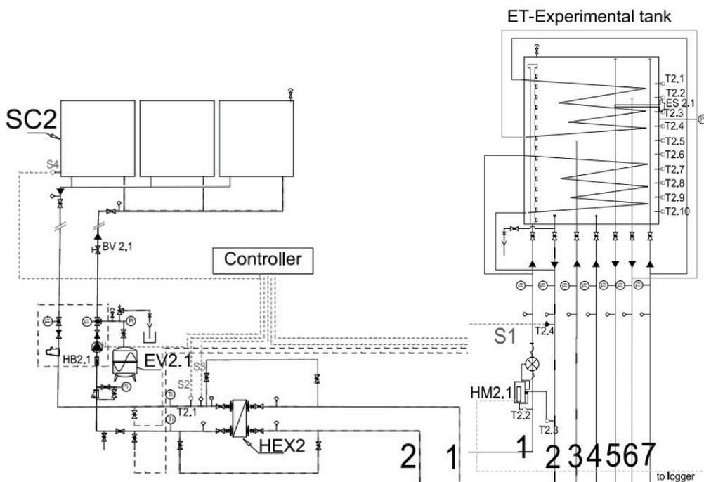
**Figure 1.** Solar collector loop on left; inlets and outlets in experimental tank (1 – hot water from HEX2; 2 – return to solar HEX2; 3 – return from heating; 4 – return from DHW; 5 – supply to DHW; 6 – return to gas boiler; 7 – hot water from gas boiler).
