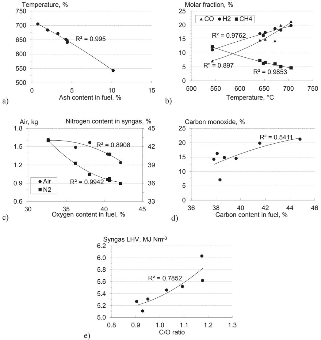
**Figure 3.** The relation between parameters in the gasification process: a) ash content in the fuel vs temperature in the gasifier reactor; b) temperature in the gasifier reactor vs CO, H<sub>2</sub> and CH<sub>4</sub> content in the syngas; c) oxygen content in the fuel vs required amount of air and nitrogen content in the syngas; d) carbon content in the fuel vs CO content in the syngas; e) C/O ratio of fuel vs produced syngas lower calorific value.
